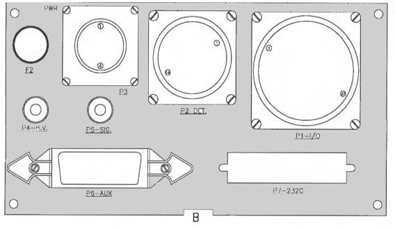
Figure 3-9. Rear Panel, Model 956A-201
