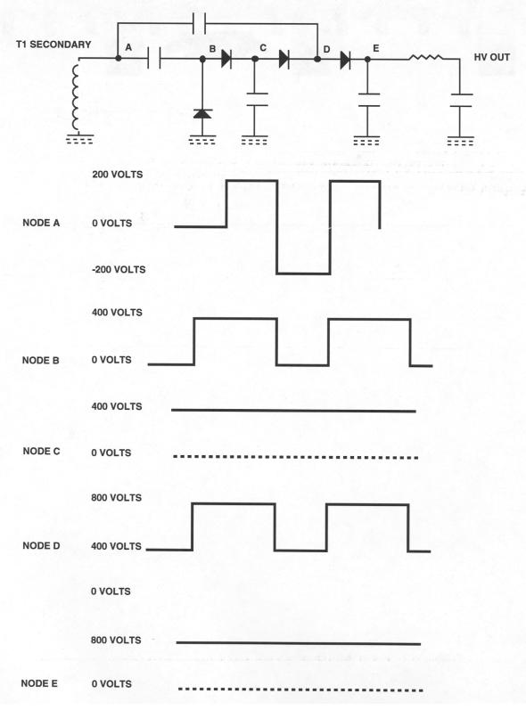
*Figure 3-7. High Voltage Output (800Vdc)*
