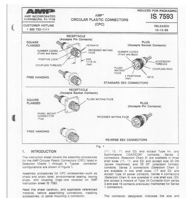
The connector designator indicates the size and contact positions of the connector. For example, 11/4 – size 11, meaning the outside diameter in 16ths of an inch as measured across the coupling threads, and contact positions 4, meaning the number of contact cavities in the connector.
