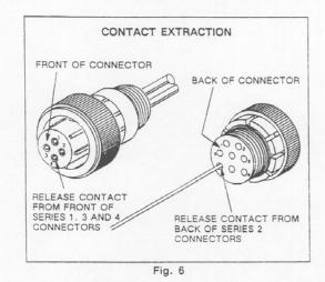
Recommendation — Socket contacts should be attached to wires leading to power source, and installed in housing that has flush mating surface. This procedure provides maximum protection for both the pin and the socket contact, and minimizes the possibility of electrical shock.
