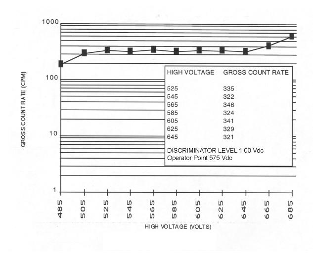
*Figure 4-1. Detector Plateau (Typical)*
