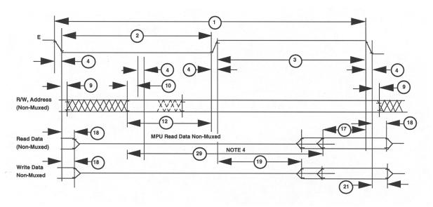
Figure 3-4. Read/Write Timing Diagram
