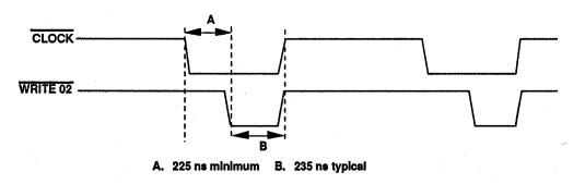
Table 3-5. Write Cycle Clock Timing Diagram
