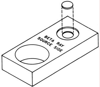
Figure 4-1. Standard Geometry Drawer Inverted to Show Recess for Beta Disk Sources
